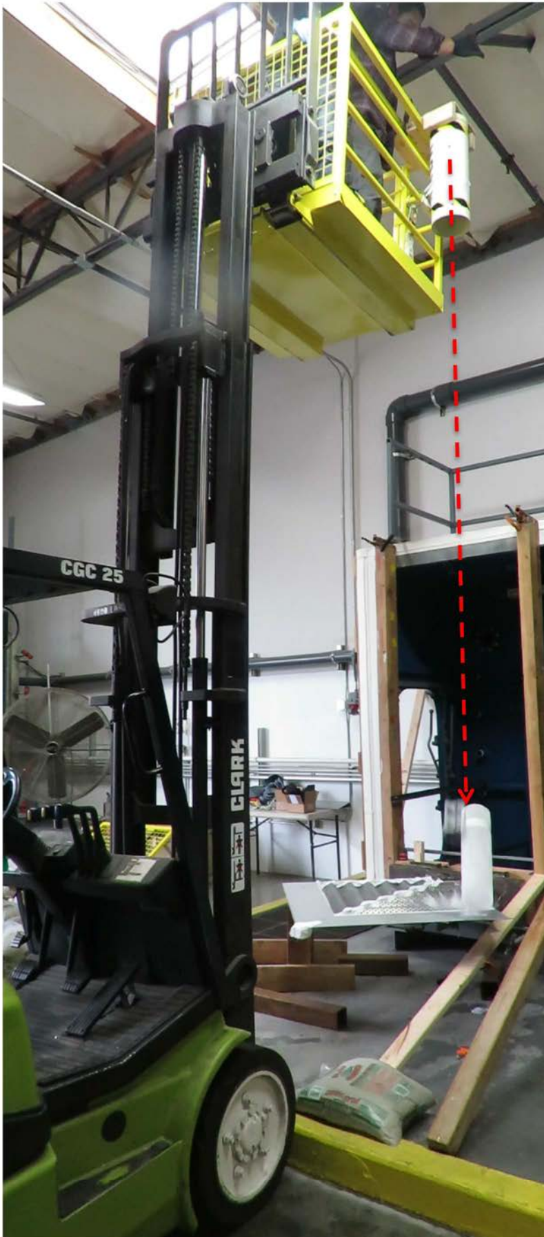
Ice impactor hitting outrigger on right end.
